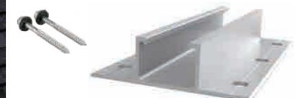
GS-IK-FR ·Description : Flat Rail Hook 1# ·Accessories : Wood screw 6.3x80 ·Spec : 120mm
